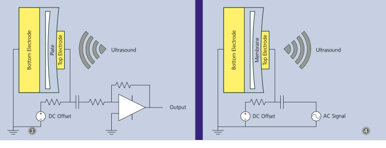
on the movable plate. This impact deflects the movable electrode generating a current between the two electrodes. This electrical current can be sensed and digitally processed to generate an image for further analysis.
